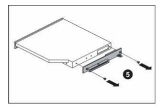
10 Using the two screws you just removed, attach the optical drive interface board to the back of the new optical drive.
